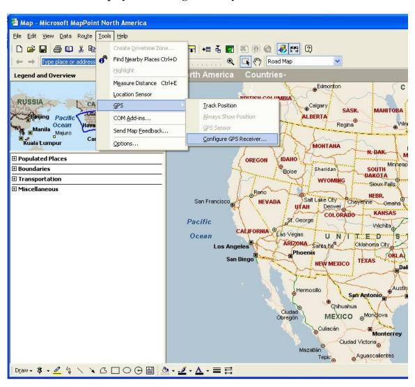
In your mapping software, go to configure your GPS device and select the comport as COM11. Then, select to track the position. You'll see the map displays of the test data. For example above, in Microsoft's Map Point, go to "tools", the GPS, then "Configure GPS receiver".
