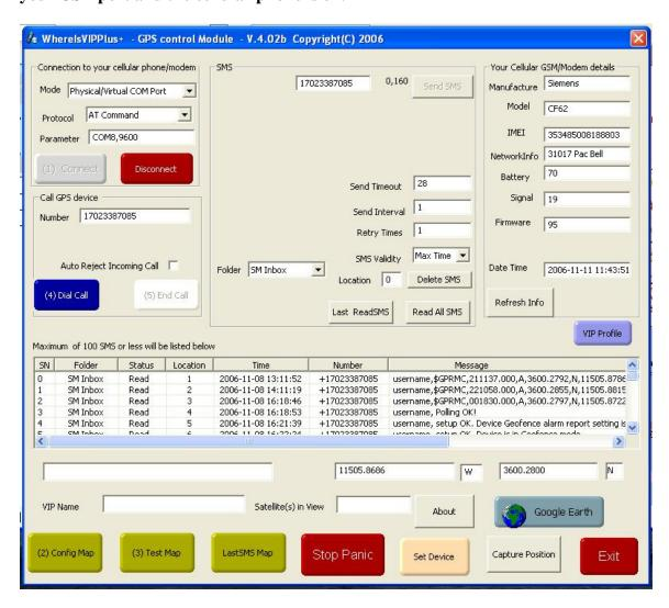
Secondly, press the Green Button "(1) connect" to begin a communication with the GSM modem/Cellular phone. The program will begin connecting with the GSM modem/Cellular phone. It will take a while and your will see the screen displays the cellular phone details including all the received SMS, as above picture.
