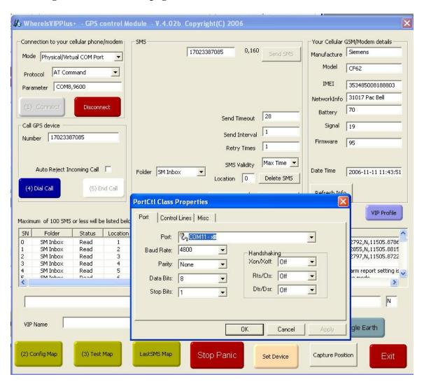
Simply, press the "(2) Config Map" button as shown above, the program will pop up a com port configuration window, click "Apply" and then "OK". Please note that if the "Apply" button is greyed-out, the port is already selected and setup.
